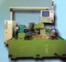
CNC銑鍵槽及倒角加工專用機 CNC keyway milling & chamfering special purpose machine
