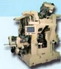
YOKE (法蘭式) 水車轉塔式加工專用機 8-station trunnion machine for yoke
