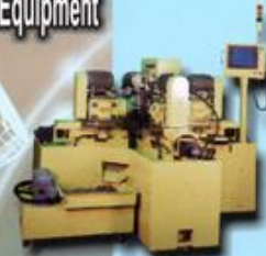
十字接頭四向倒角加工專用機 4 side chamfering machine for universal joint
